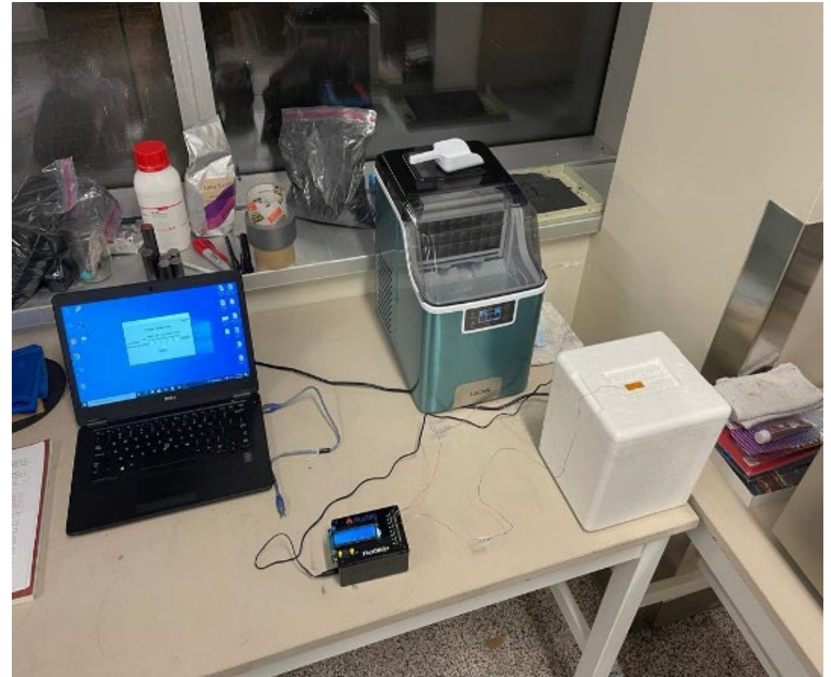
Complete system set-up (Ice maker, FluxTeq, Cooler, Simulation)
