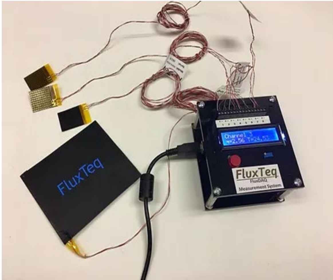
Heat flux and temperature measurement devices from FluxTeq
