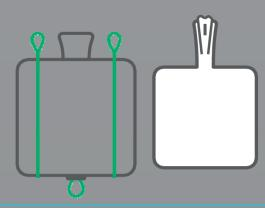
Cubic shape optimizes space Retains cube shape for easy stacking Reduced risk of punctures and snags Very strong – constructed with 5x safety factor
