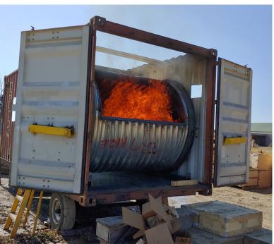
Above and below: 72-inch (6-ft, or 1.8 meter) RoCC kiln inside a 20-ft shipping container w/ mechanical rotation
