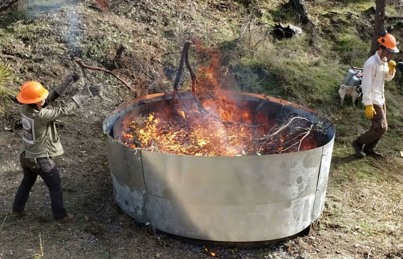
Biochar production in a Ring of Fire kiln, piloting hot-loading with green material.
