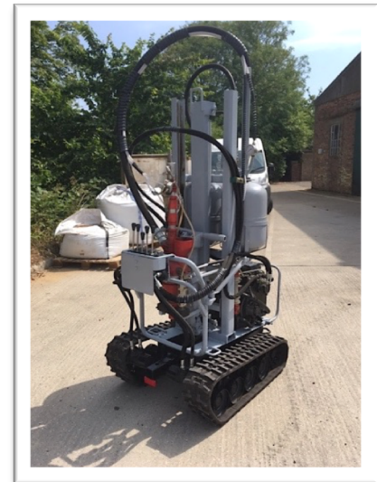
Figure 6 - Terra Aeration Tracker Pneumatic Soil Decompaction (Source: Terra Aeration)
