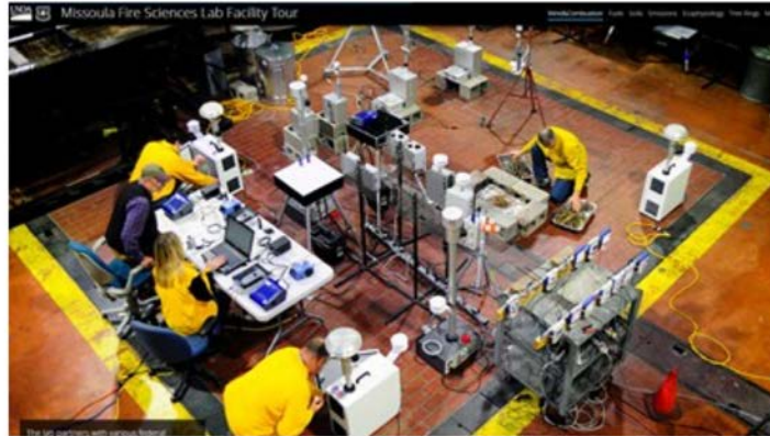
USFS Missoula Fire Lab's Combustion Chamber floor and sampling hood that will be used for this study's emissions testing in the laboratory.
