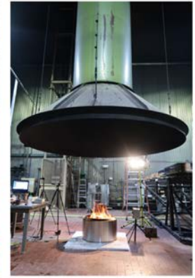
USFS Missoula Fire Lab's Combustion Chamber floor and sampling hood that will be used for this study's emissions testing in the laboratory.
