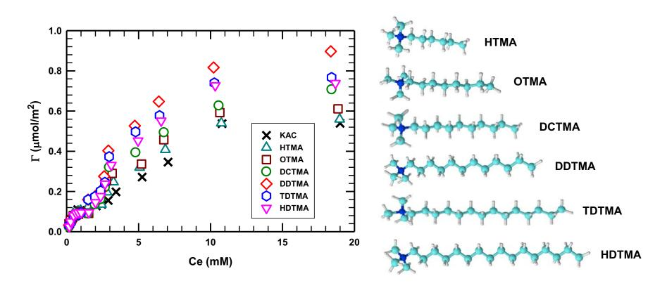
Adsorption of fluoride on KAC functionalized HTMA, OTMA, DCTMA, DDTMA, TDTMA, and HDTMA.
