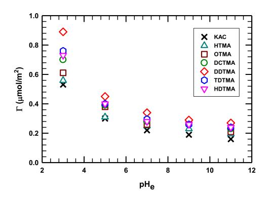
Effect of pH on fluoride removal by functionalized KAC functionalized with HTMA, OTMA, DCTMA, DDTMA, TDTMA, and HDTMA. Experimental conditions: [FAC] = 2 g/L, I =  $10^{-2}$  M NaCl. AC modified with 10 mM of Quats.
