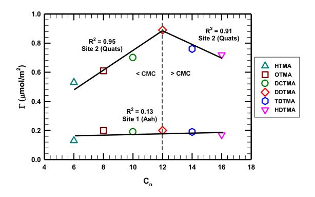
Adsorption of fluoride on KAC functionalized with HTMA, OTMA, DCTMA, DDTMA, TDTMA, and HDTMA.
