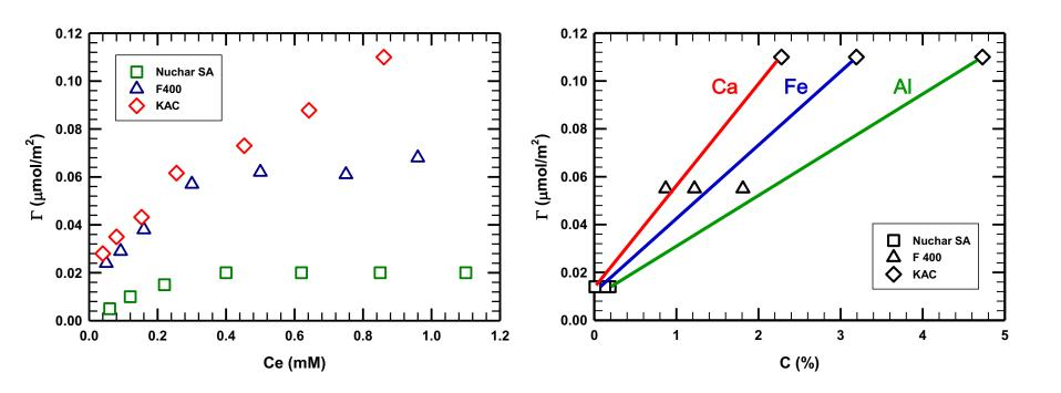
Effect of ash composition for fluoride removal by plain activated carbon. Experimental conditions: [AC] = 2 g/L,  $I = 10^{-2} \text{ M NaCl}$ , pH = 7.
