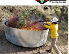
The Ring of Fire Kiln by Wilson Biochar is an easily-portable, modular kiln designed for use by hand crews. It can be deployed in hard to reach locations off-road in forests and on farms.
