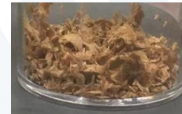
Lignin extraction for 18 hr at 140 °C
