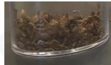
Lignin extraction for 2 hr at 140 °C
